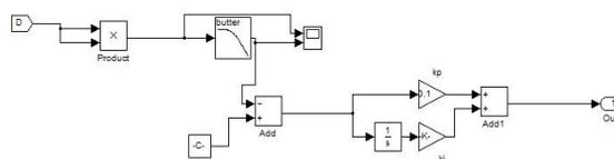
Figure 5: MATLAB/SIMULINK diagram of fast acting dc controller.
