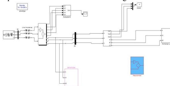
Figure 8: MATLAB/SIMULINK diagram of DSTATCOM at distribution station with non linear loads.
