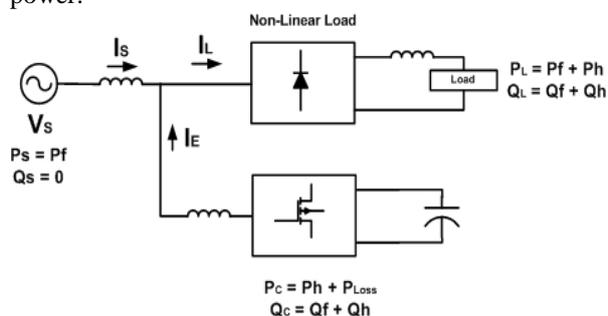
Figure 1: Basic two levels VSC based DSTATCOM.
