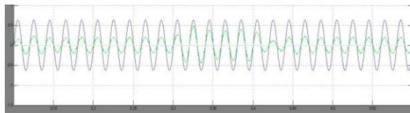
Figure 18: Phase A Voltage in phase with current.
