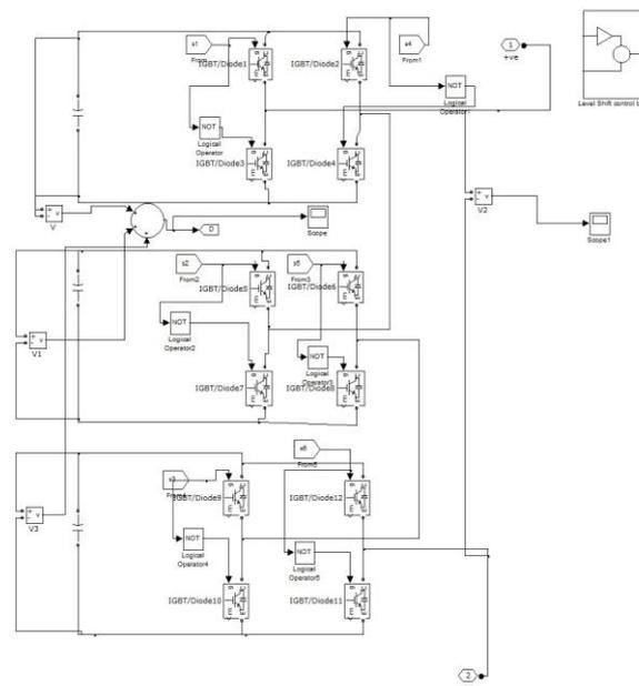
Figure 2: Seven level Cascaded H-Bridge Inverter per phase in DSTATCOM.
