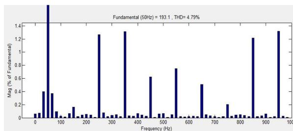
Figure 13: THD value in line current of seven level-shift PWM CHB inverter.
