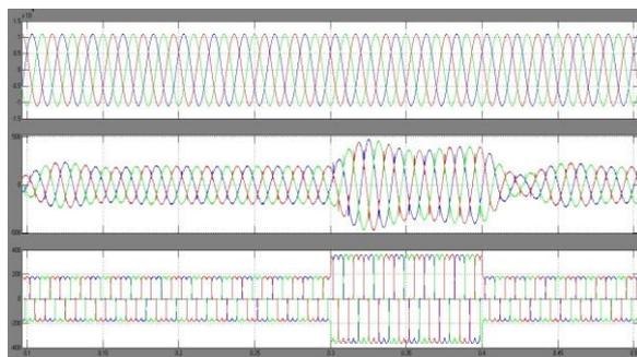
Figure 12: With DSTATCOM seven level- Level shift PWM technique of CHB inverter results 1) Source Voltage 2) Source current & 3) Load current.
