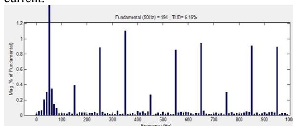
Figure 16: THD value in line current of seven level-shift PWM CHB inverter.
