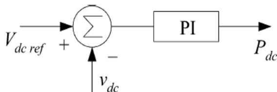
Figure 3: Schematic diagram of the conventional dc-link voltage controller.
