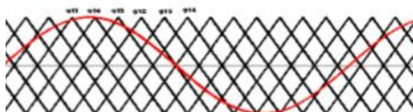
Figure 6: Phase shifted PWM for seven level CMC.
