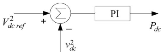
Figure 4: Schematic diagram of the fast-acting dc-link voltage controller.
